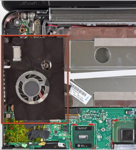
*(i)* If present, remove the large piece of black adhesive film covering the area around the fan.
